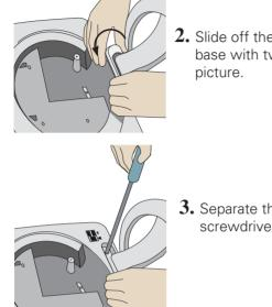
2. Slide off the lower section of the cover base with two hands as shown in the
